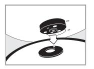
Position the magnetic wheel onto the magnetic adaptor on the projector. To remove the wheel simply lift it off.
