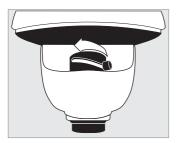
To focus the projected effect, twist the slide on the lens forward and backwards until your desired focus is achieved.
