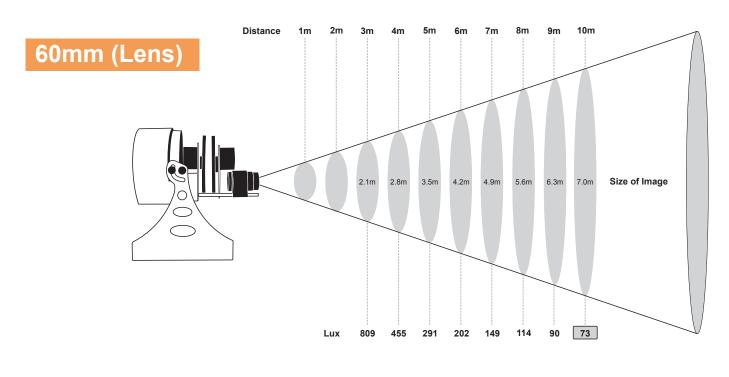
Ratio for Distance 1,4:1 (Image Size - 60mm Lens) no other light sources nearby The Object Diameter is 42mm
