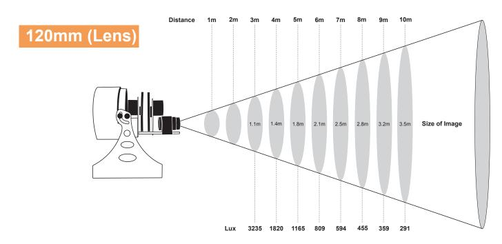
Ratio for Distance 2,9:1 (Image Size - 120mm Lens) The Object Diameter is 42mm
