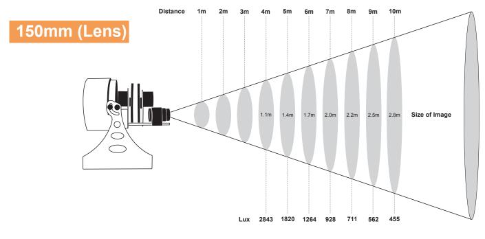
Ratio for Distance 3,6:1 (Image Size - 150mm Lens) The Object Diameter is 42mm
