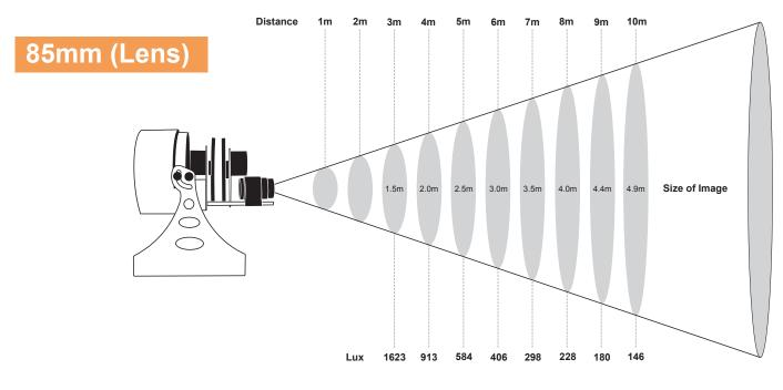
Ratio for Distance 2:1 (Image Size - 85mm Lens) The Object Diameter is 42mm
